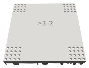
Figure 11. Bottom side of a final section where both the label and the grid of cylinders are inserted
