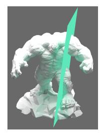
Figure 8. Cut one part of a geometry which is not self-supported
